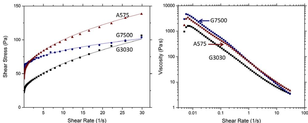
**Fig. 5.** Flow curves for silicon nitride suspensions with 43 vol% solids loading and 5 vol% dispersant content for the three studied dispersants. Curve fits to the Herschel–Bulkley fluid model are shown as solid lines with  $R^2 > 0.99$ . Viscosity as a function of shear rate shows a shear thinning trend for all three dispersants.
