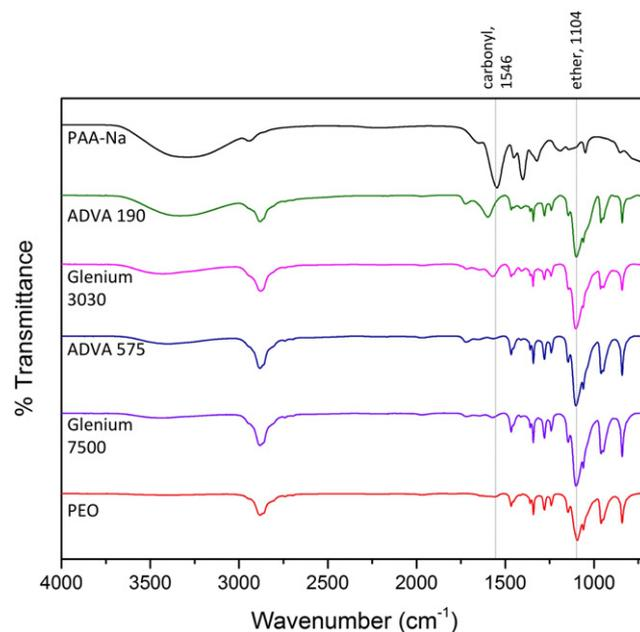
Fig. 2. FTIR spectra of the four WRAs studied along with reference spectra for PEO and a sodium salt of PAA (PAA-Na). The strong peak around 1550  $cm^{-1}$  can be attributed to the C=O (carbonyl) stretch in PAA-Na, while the peak around 1100  $cm^{-1}$  can be assigned to the C–O–C (ether) stretching hydrating bond in PEO. The ratio of the area under these peaks is used to analyze the PAA-Na/PEO peak ratio.
