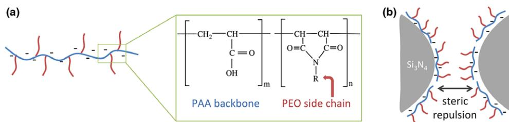
**Fig. 1.** Schematic illustration of (a) molecular structure of typical comb polymer water-reducing admixtures composed of PAA backbones with PEO side chains ( $\text{R} = (\text{CH}_2\text{CH}_2\text{O})_x\text{-CH}_3$ ) and (b) coating of  $\text{Si}_3\text{N}_4$  particles with charged PAA backbone and PEO side chains providing steric repulsion between particles to stabilize the suspension (not drawn to scale).
