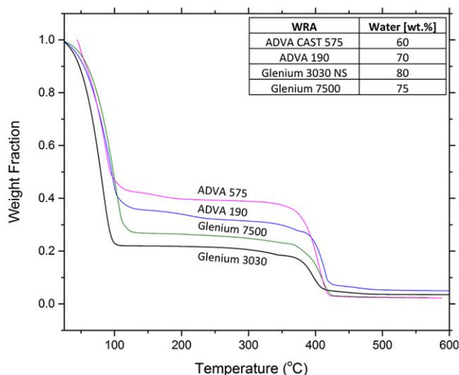
**Fig. 3.** Weight loss as a function of temperature results for dispersants as obtained via thermogravimetric analysis experiments in a flowing nitrogen atmosphere. The water content in each dispersant was quantified by measuring the weight loss upon heating from 25°C through the plateau in mass loss. Mass loss typically started at 100°C and continued through 400°C. All four samples reached >97% weight loss by approximately 420°C.
