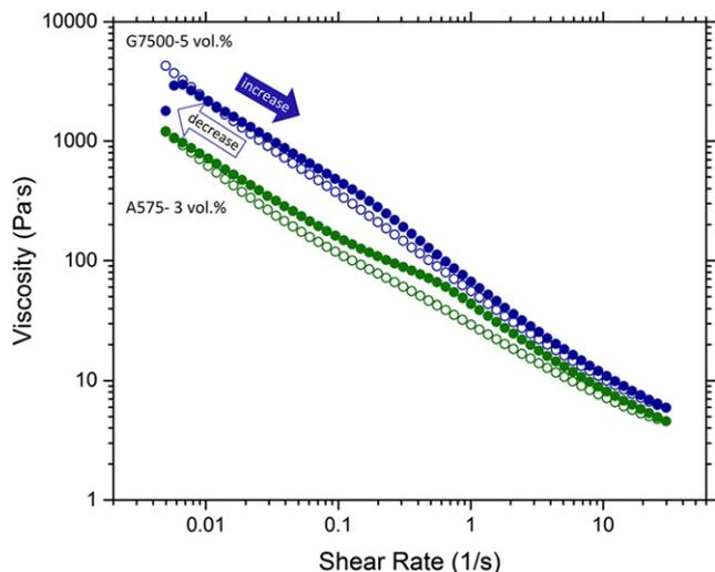
**Fig. 10.** Viscosity as a function of applied increasing, followed by immediate decreasing, shear rate for optimized 45 vol% suspensions using both Glenium 7500 and ADVA 575 as dispersants. G7500 shows little to no thixotropic behavior due to the small gap between viscosity for increasing and decreasing shear rates, while A575 shows a larger gap and therefore slightly more thixotropic behavior.
