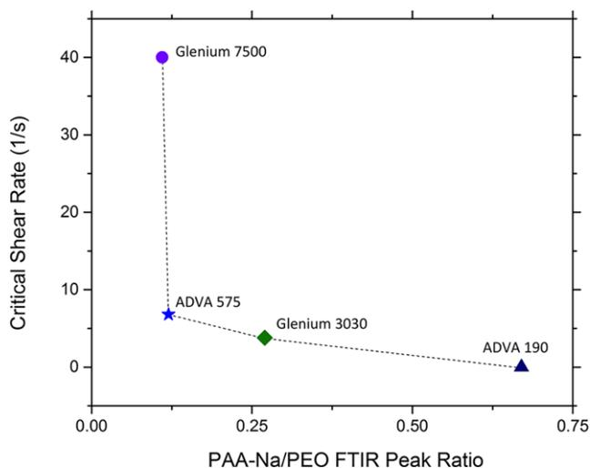
**Fig. 7.** Critical shear rate where suspensions exhibit onset of shear-thickening behavior as a function of PAA-Na/PEO peak ratio (determined via FTIR). The dotted line shown is simply to direct the eye.
