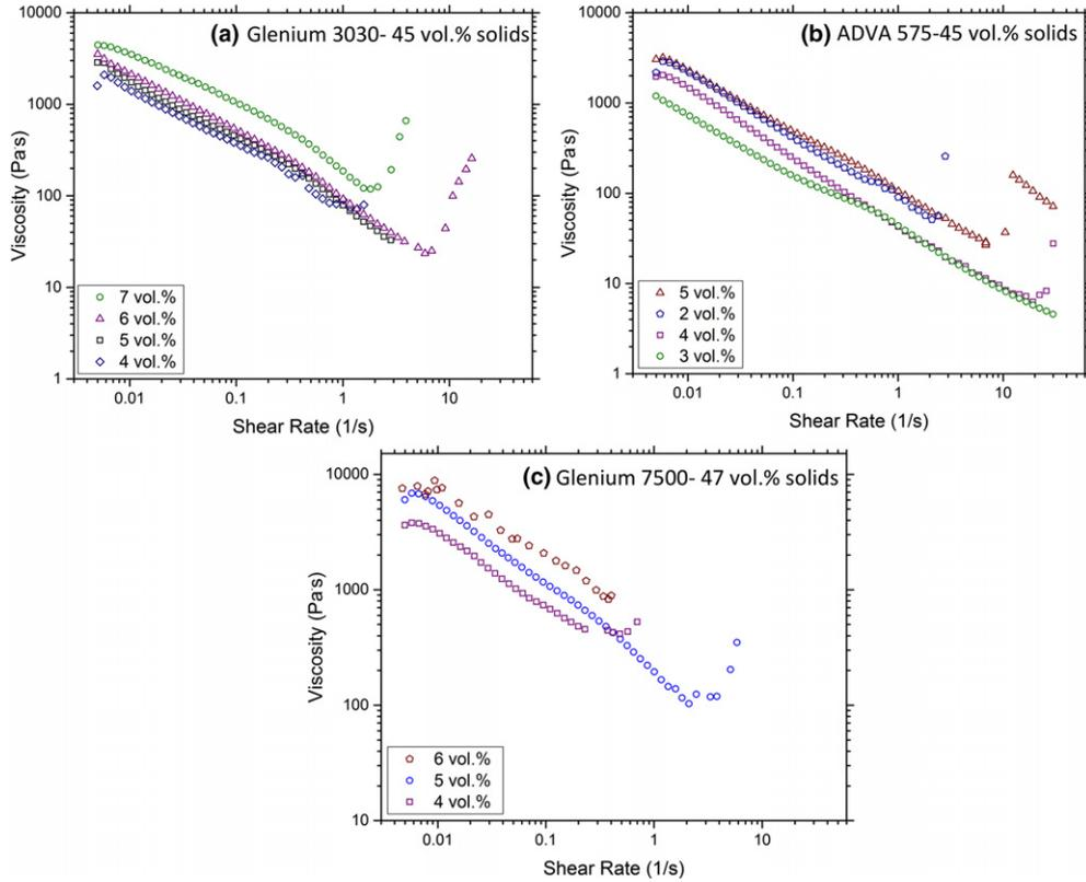
**Fig. 8.** Viscosity as a function of shear rate for suspensions with 45 vol% solids loading and varying dispersant content for (a) Glenium 3030 and (b) ADVA 575. Optimization for (c) Glenium 7500 was done with 47 vol% solids loading in order to see the critical shear rate in the shear rates studied. The optimal dispersant content is chosen as the suspension with the largest critical shear rate.
