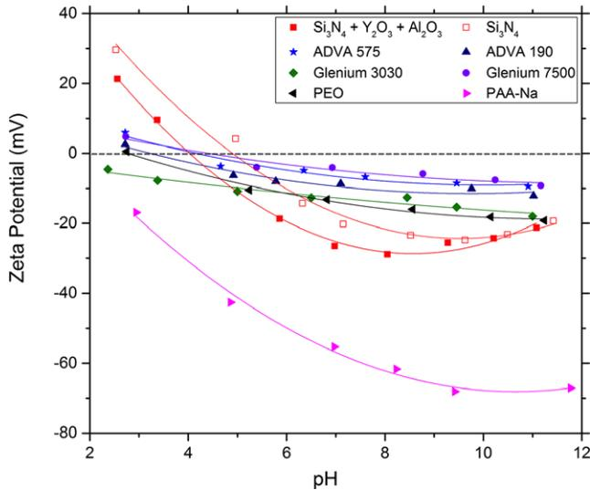
**Fig. 4.** Zeta potential of as-received  $\text{Si}_3\text{N}_4$  powder and with 5 wt%  $\text{Y}_2\text{O}_3$  and 5 wt.%  $\text{Al}_2\text{O}_3$  added as sintering aids in water and with polymer dispersants. Studies with dispersants were conducted with the sintering aid mixture. Solids loading of 0.05 wt% ceramic powder was used for all studies, with 0.025 wt% dispersant used with respect to the total mass of the sample.
