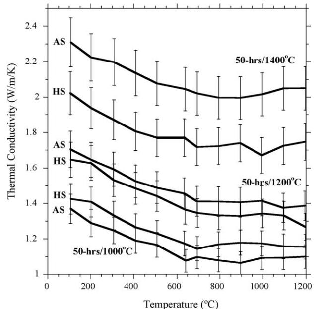
Fig. 4. Thermal conductivity of stand-alone as-sprayed and heat treated after 50 h heat treatments at 1000, 1200 and 1400 °C for coatings made from AS and HS powders. From graph bottom to top, the first and second lines represent the thermal conductivity after 50 h heat treatments at 1000 °C, the third and fourth lines represent the thermal conductivity after 50 h heat treatments at 1200 °C, and the fifth and sixth lines represent the thermal conductivity after 50 h heat treatments at 1400 °C.
