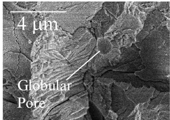
Fig. 2. SEM micrograph of the cross-section of an as-sprayed coating made from AS powders.
