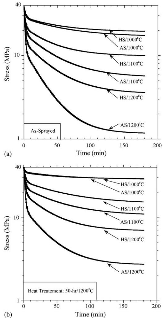
Fig. 5. (a) Comparison of stress–relaxation behavior of stand-alone as-sprayed coatings made from AS and HS powders as a function of test temperature. The initial stress in each coating was 40 MPa; (b) comparison of stress–relaxation behavior of stand-alone heat-treated coatings made from AS and HS powders as a function of test temperature. All heat treatments were conducted for 50 h at 1200 °C prior to testing. The initial stress in each coating was 40 MPa.
