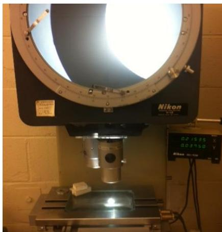
Figure S2. Nikon Profile Projector V-12 used to measure the diameters of o-ring seals before and after immersion in neat and doped Sasol IPK.
